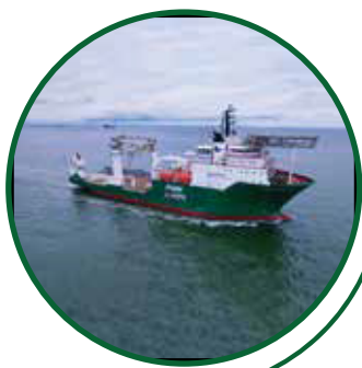
Offshore Construction Vessel DP3/250T AHC Crane
