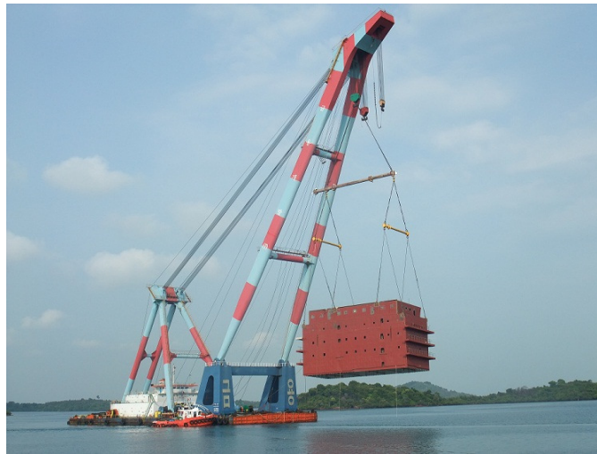
Floating Sheerleg 800T Lift Capacity
